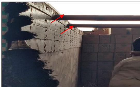
Type 1- Fixed horizontal Angles in a truck creating issue while loading the top layer. It reduces the material carrying capacity of the vehicles.
