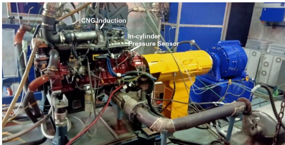
Fig 5.21: Test engine's CNG fuel induction and mounting position of In-Cylinder Pressure Sensor.
