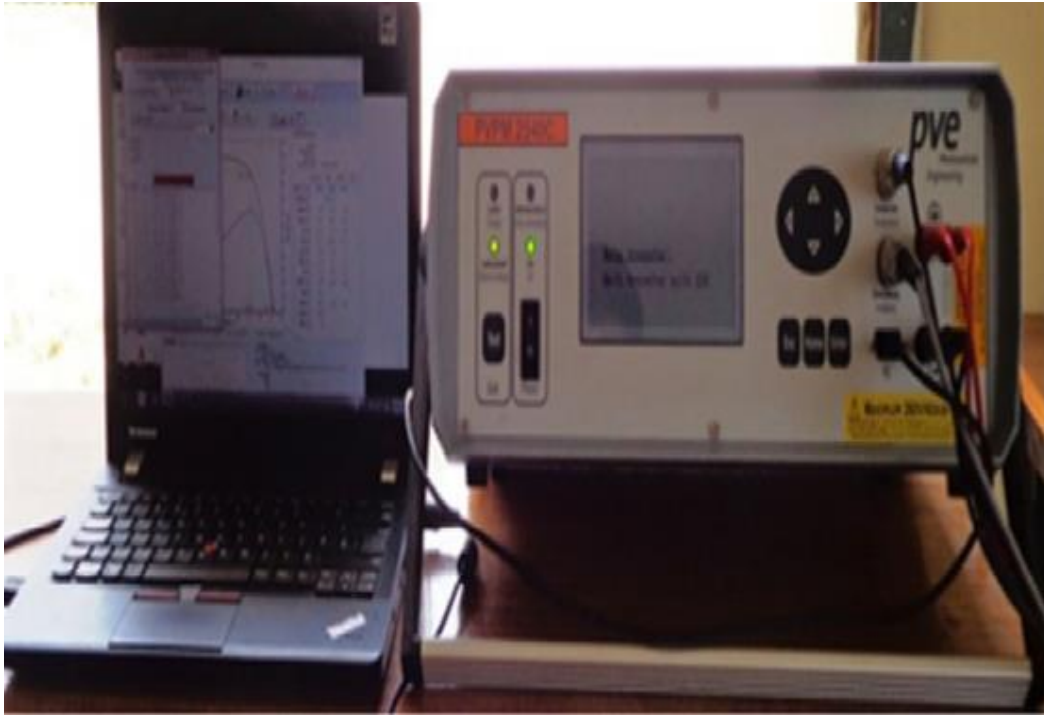
Figure 3.10 I-V Tracer and data stored in PC
