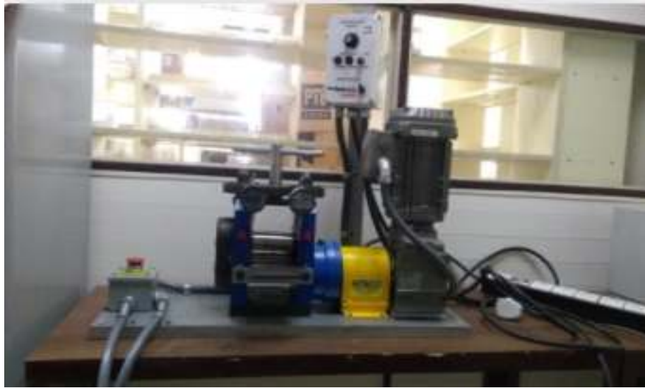
Fig. 3.2 (b) Rolling Machine 1 at IUAC
