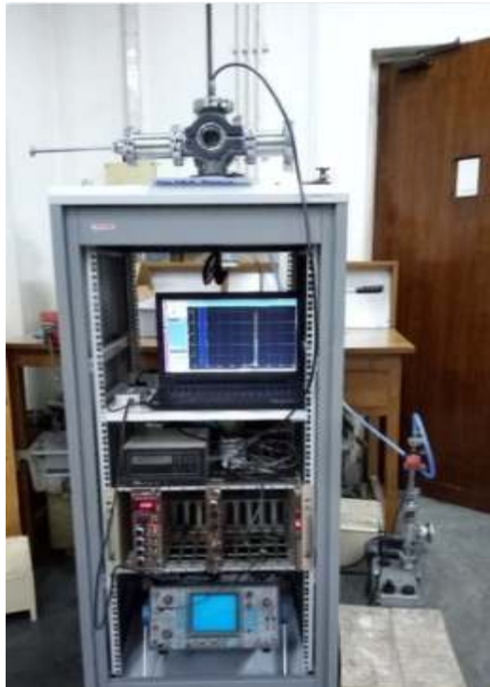
Fig. 3.5. \alpha -spectroscopy thickness measurement set-up at Target Laboratory, IUAC
