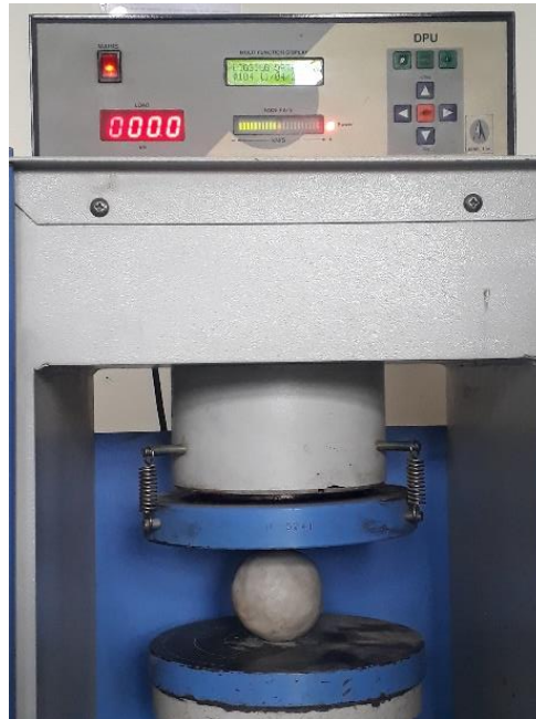
Figure 5-19 Compression test of storage material
