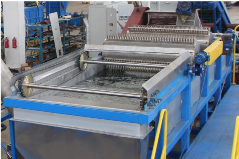
Figure 2-12 Sink and Float separation tank by Amster Machinery Co., Ltd. (Amstar Machinery, n.d.)
