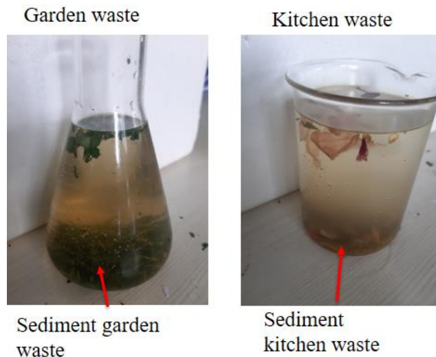
Figure 4-2 Behavior of kitchen and garden waste in water
