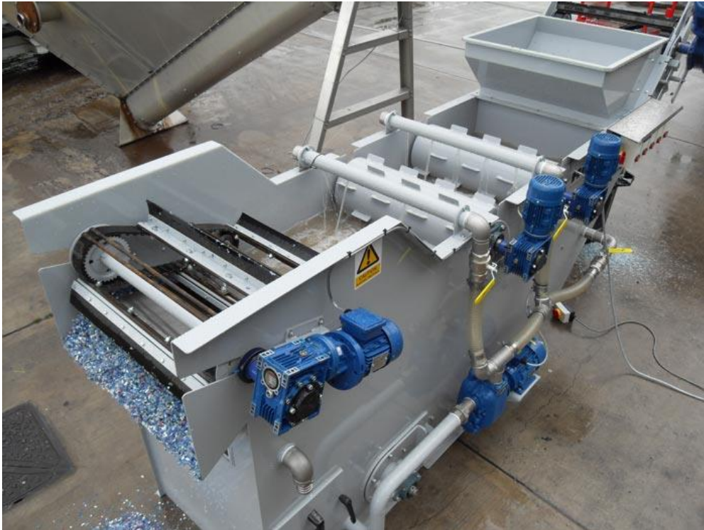
Figure 2-11 Sink and Float separation tank by Haith group (Haith Group, n.d.)
