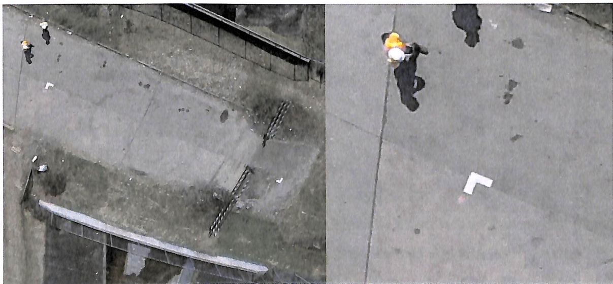
Figure 3: Example of Ground Control Points Viewed from a UAS
