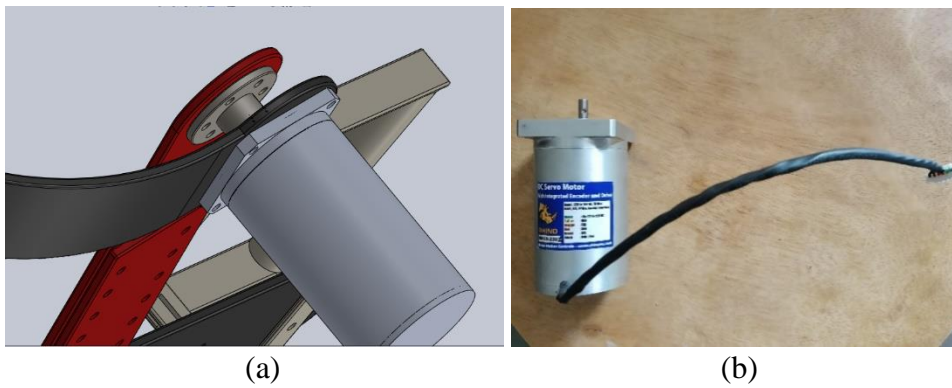
Figure 5.6 (a) CAD model and (b) Actual Rhino DC servo motor
