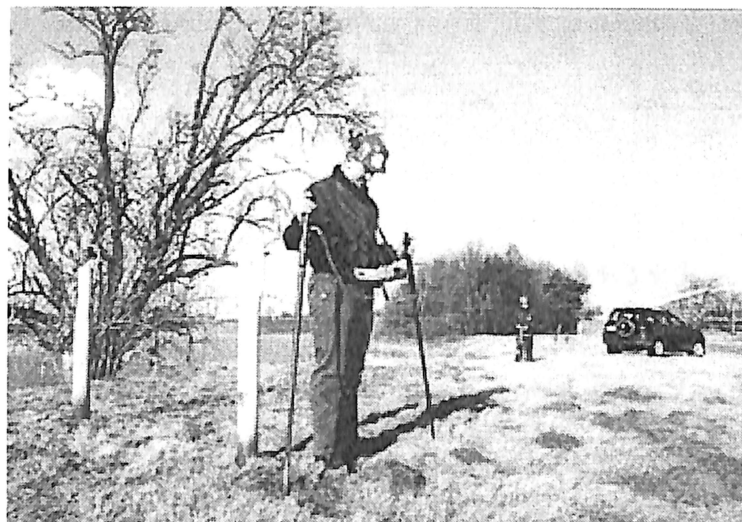
Fig. 3.4 DCVG Survey technique
