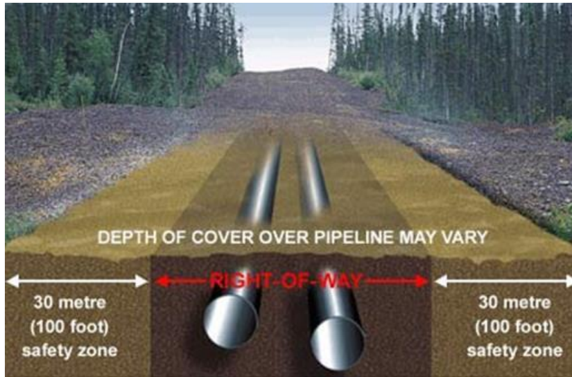
Fig A-11: A typical Awareness Notice in Pipeline ROW for Sensitizing people,
