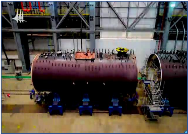
Fig 15 :- Submarine Cutsections for AIP Plug fitment at construction yard
