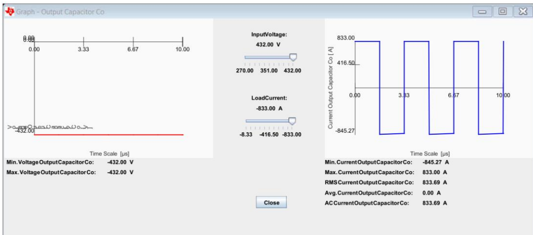
Fig 5.49: Waveforms at Output capacitor Co – 432 Volts
