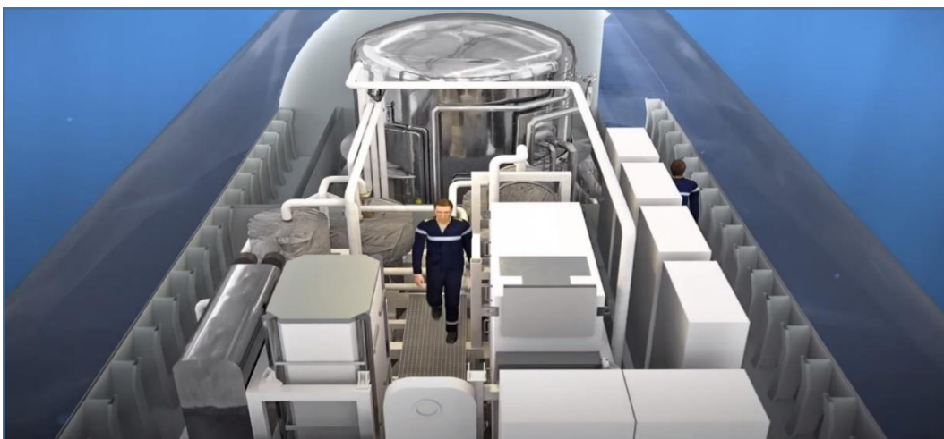
2.46: Top view of 3D-modelled Diesel Reforming system onboard submarine[249]
