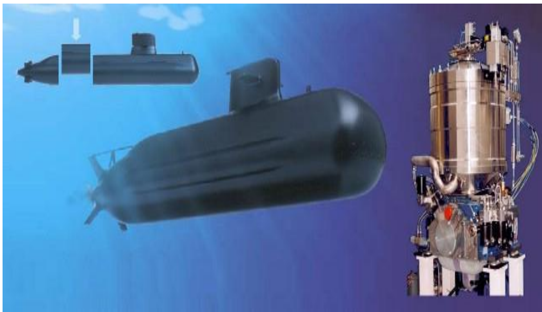
Fig 2.30. Stirling Engine AIP system [237]
