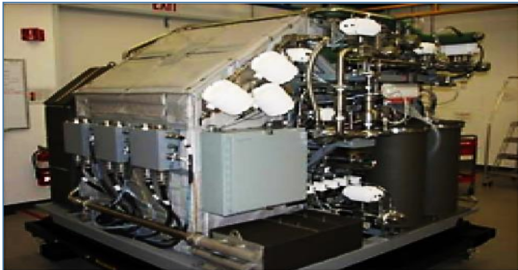
Fig 2.39: Land Based Setup of bio-Ethanol fed AIP system of S-80 Submarine[243]
