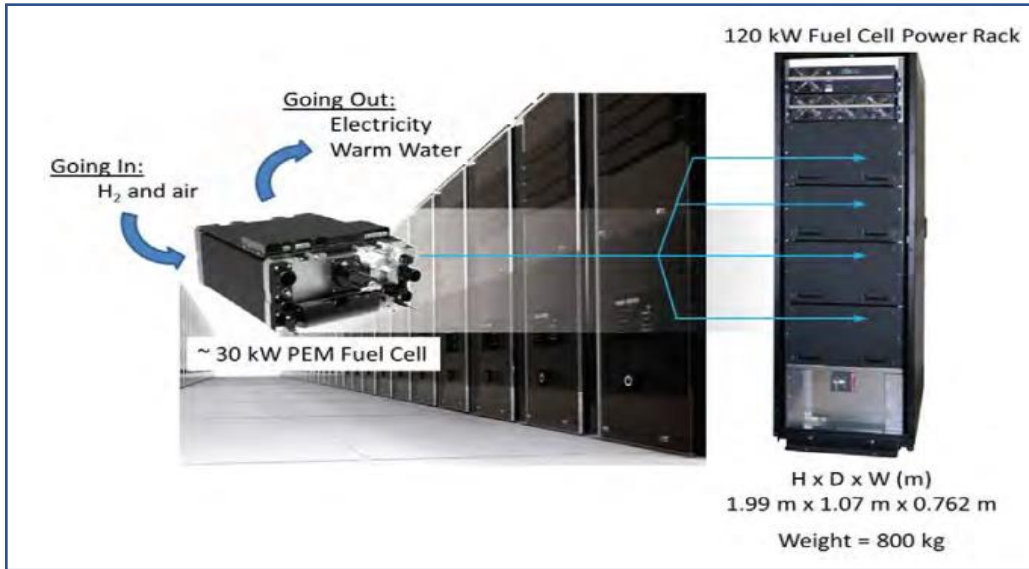
Fig 5.30: HyPM-R-120S PEM Fuel Cell Rack with Dimensional details
