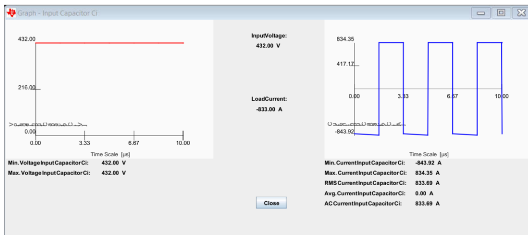
Fig 5.43: Waveforms at input capacitor – 432 Volts
