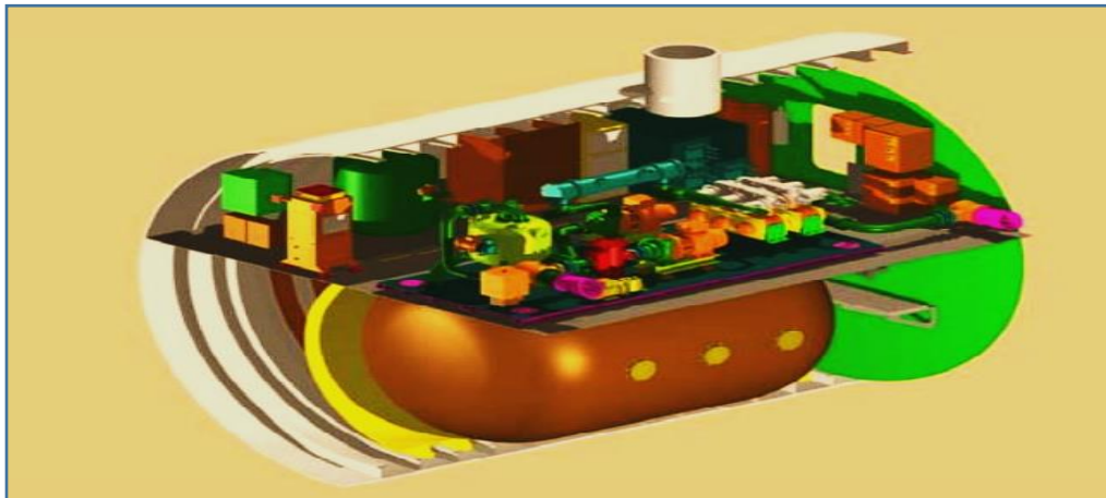
Fig 2.40: Graphical representation of Methanol reforming AIP Fuel cell plug of Spanish S-80 Program[244]
