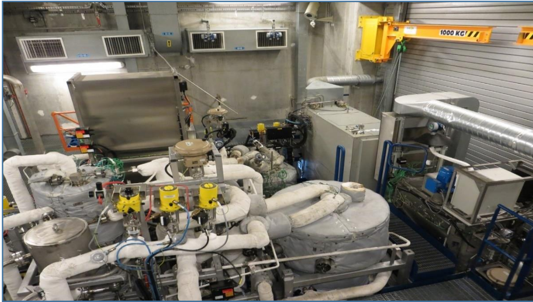
Fig 2.45: laboratory setup of Diesel reforming AIP system of M/s DCNS, France [249]
