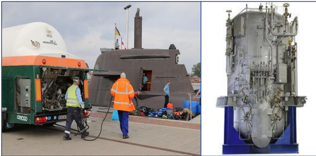
Fig 5.50 (Left to right): (a) Refueling of LOX onboard an AIP Submarine[249]. (b) LOX storage container of M/s Air Liquide, France for AIP Submarines[374].
