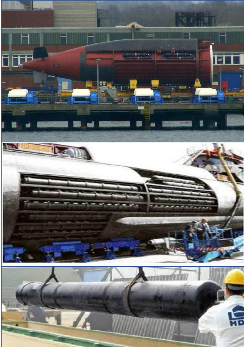
Fig 5.53 (Top to bottom): (a) Aft portion-Cut Section of German Type 212 on syncrolift showing Metal Hydride tanks around pressure hull during construction, Kiel , Germany [378] (b) Wholly booted Type 212A submarine [379] (c) Metal hydride cylinder being removed by crane for maintenance [33]
