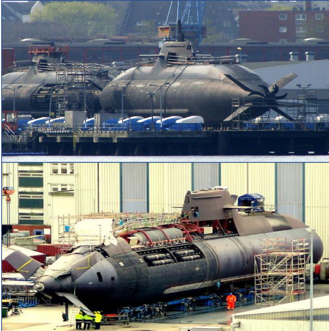
Fig 5.52 (Top to bottom): (a) German Type 212 on syncrolift [376](b) German AIP Submarine with Metal hydride and LOX storage tanks on pressure hull[377].
