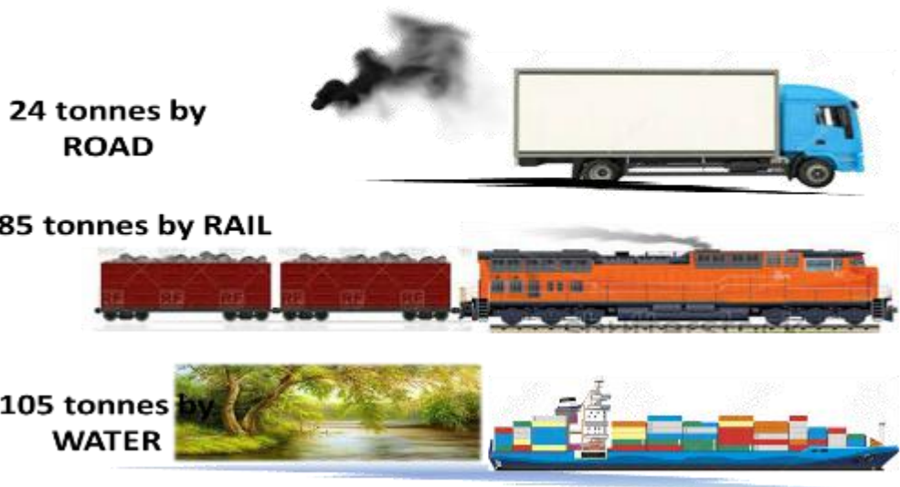
Figure 1.1 Fuel efficiency of Water mode as compared to Rail and Road (Author)
