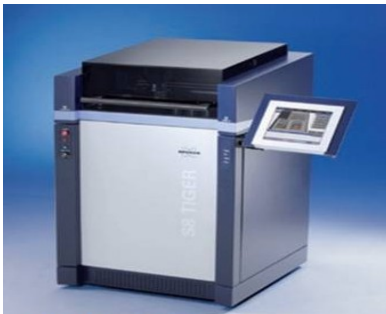
Figure 3.3 Wavelength dispersive X-ray Fluorescence (WDXRF) Spectrometer for analyses of the major and trace elements (at WIHG).
