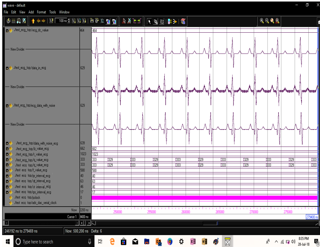
Fig.6.21 ECG signal with P, Q, R, S and T values
