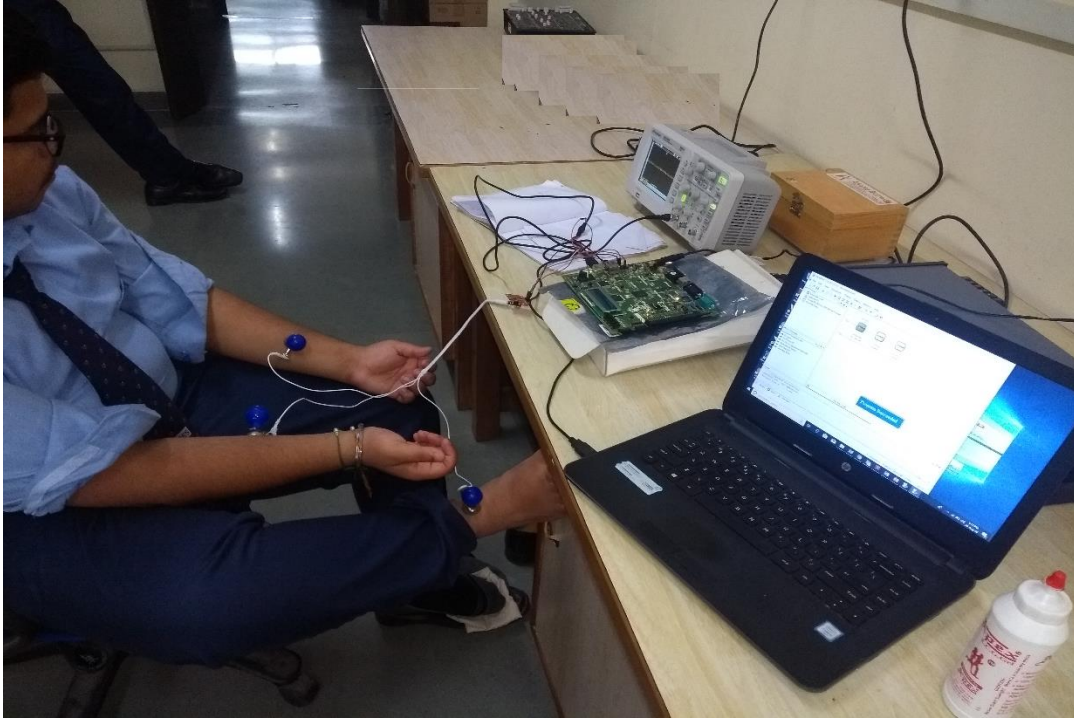
Fig. 7.4 ECG real time ECG signal processing set-up
