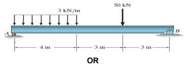
For the beam and loading shown in figure below, draw SFD and BMD. Using Mohr's area moment method, determine the deflection of the point at a distance 0.5 m from point A for the loaded beam. Take EI =  $8.3 \times 10^5 \text{ Nm}^2$ . (CO2)
