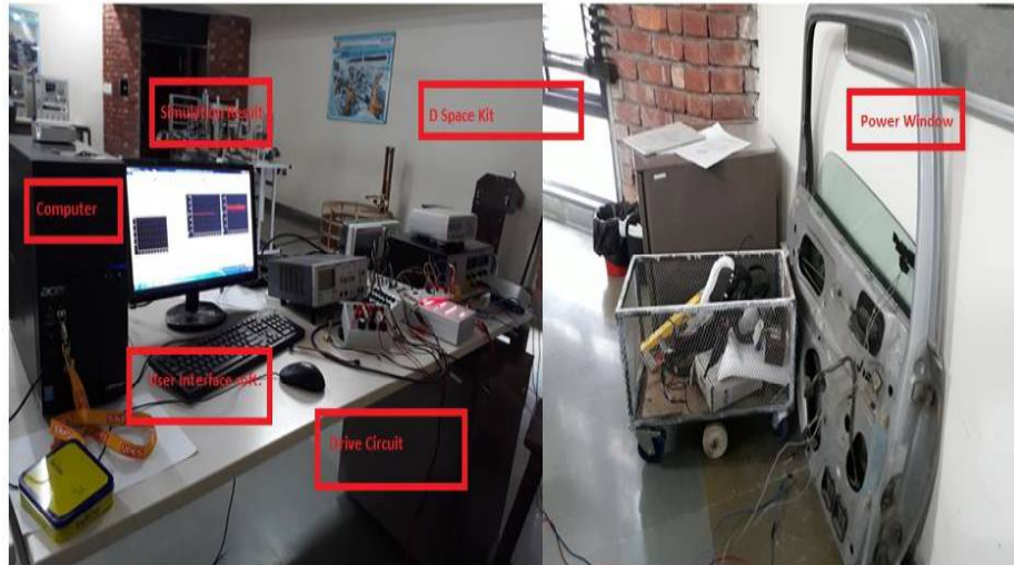
Figure 3-11 Test Bench setup of power window system with dSPACE Kit.
