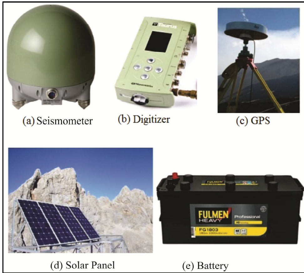
Figure 3.1 Components of a seismograph system (a) seismometer (b) DAS (c) Global Positioning System (GPS), power supply unit comprising (d) solar panel and (e) battery.
