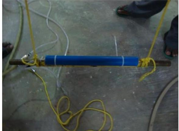
Fig 5.4: Pespex pipe assembly connected to 3/4<sup>th</sup> inch air hose with rope and mounting arrangement with dead weight.
