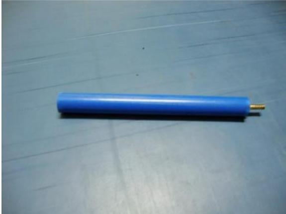
Fig 5.3: Pespex pipe of 2inch diameter and 12 inches length with 1inch aperture with 3/4<sup>th</sup> inch brass gas inlet nozzle.
