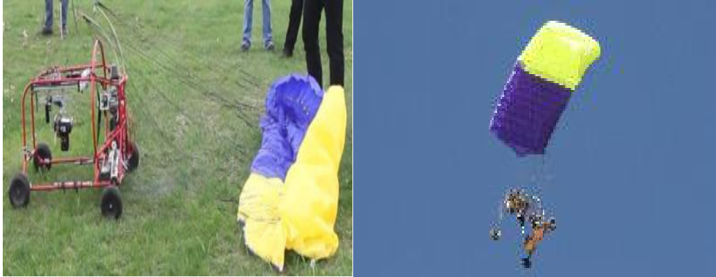
Figure 1.3. A Powered Parafoil UAV [2]
