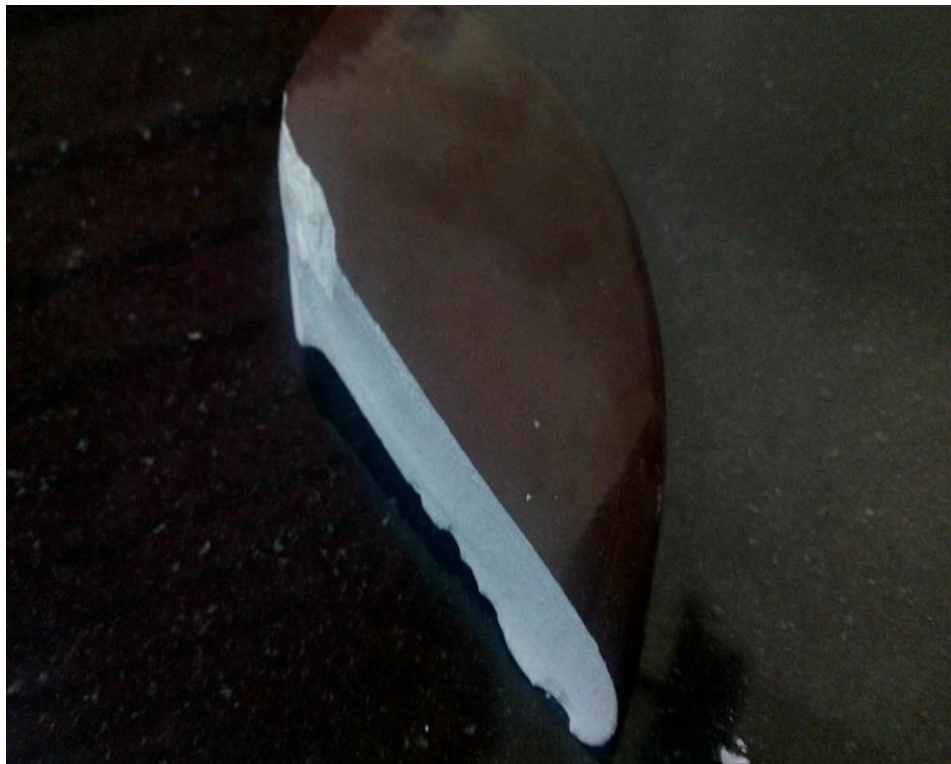
Figure 5-8: Broken porcelain insulator during rain test
