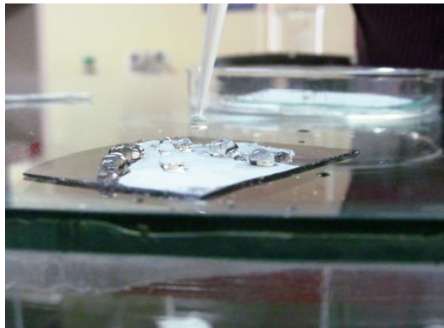
Figure 4-11: Water droplet on a nano powder coated silicon water
