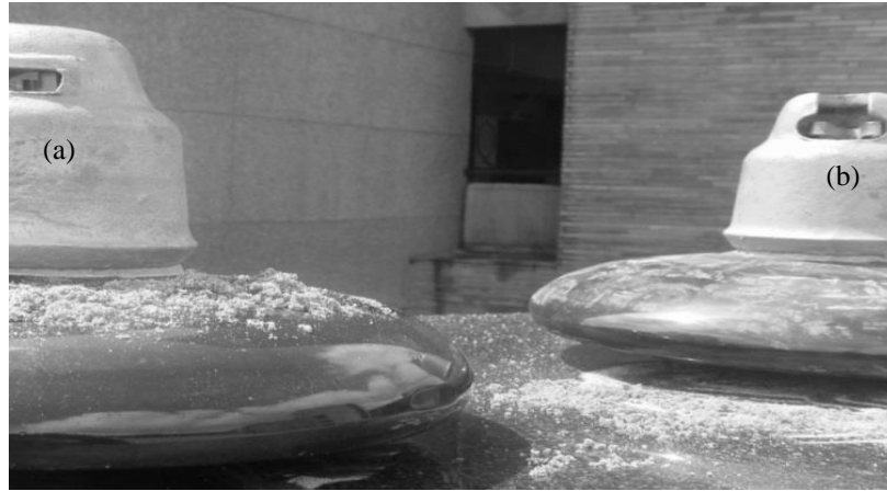
Figure 5-9: (a) uncoated insulator with deposition of mist and dust still on the surface. (b) nano coated insulator with all the deposition of mist and dust roll off from the surface of the insulator.
