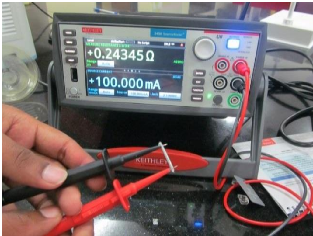
Figure 4-2: Aluminum conductor without coating indicating resistance.
