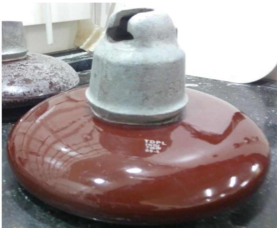
Figure 5-1: Uncoated insulator post insulator bushing of 70kN from Tehri Distribution Power Limited, Power Transmission Corporation of Uttarakhand Limited.
