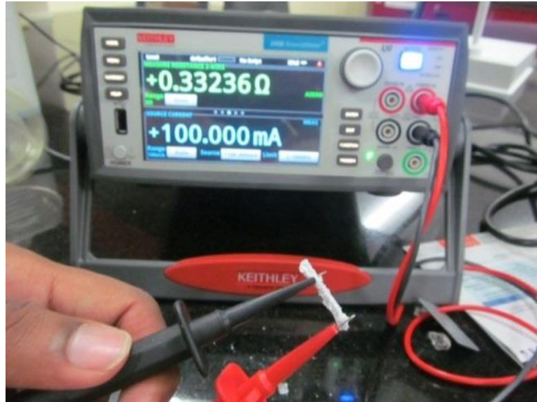
Figure 4-3: Aluminum conductor showing the increase of resistance value.
