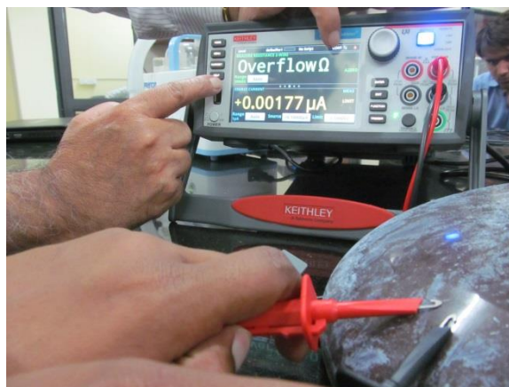
Figure 3-5: The picture above showing the open circuit condition, hence no leakage currents.
