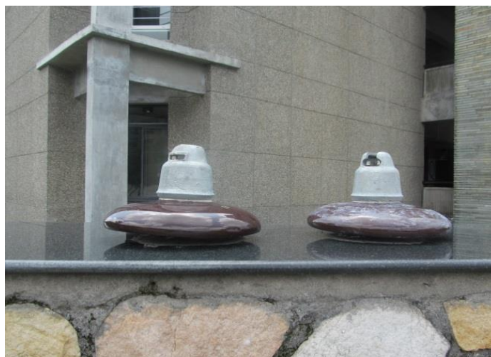
Figure 4-15: Coated and uncoated porcelain insulator kept in atmospheric conditions for dusty layer formation
