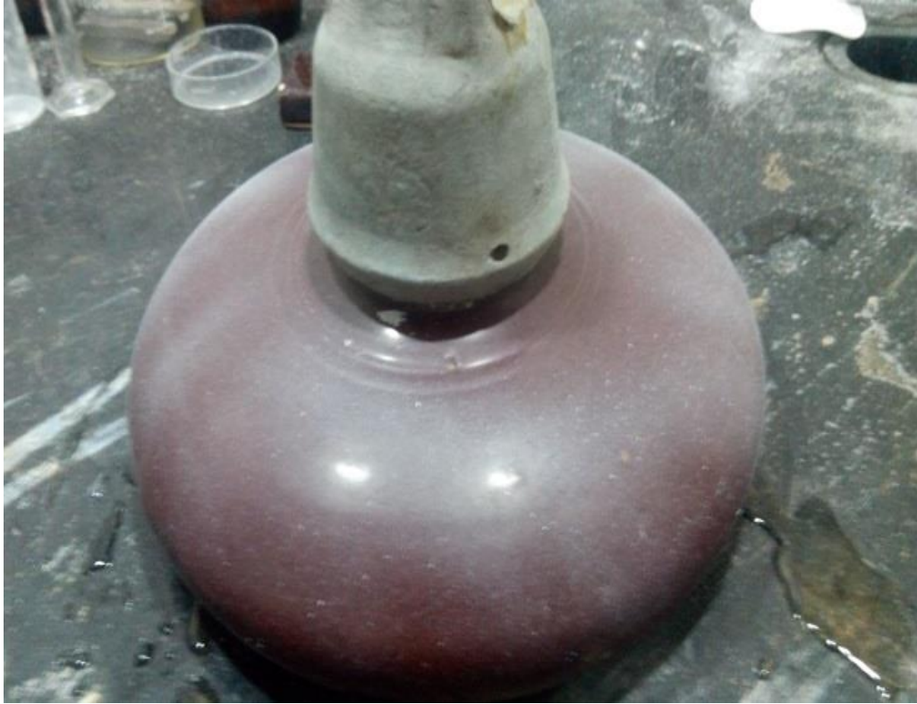
Figure 5-6: Coated insulator without any dust particle
