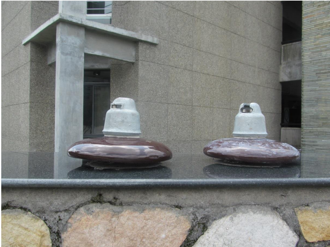
Figure 5-4: Coated and uncoated insulator is kept for observation in a commercial building construction polluted area.
