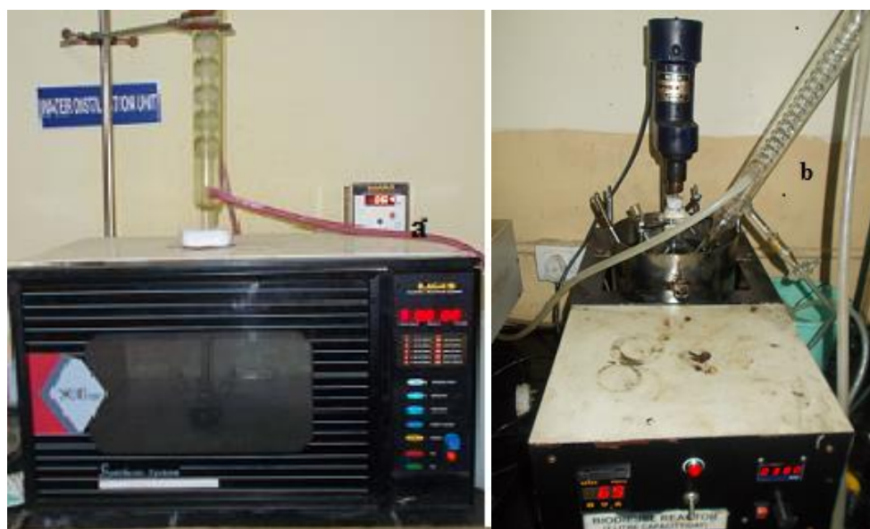
Figure 3.16 Experimental set up used for transesterification, (a) microwave assisted transesterification reactor, (b) conventional transesterification reactor
