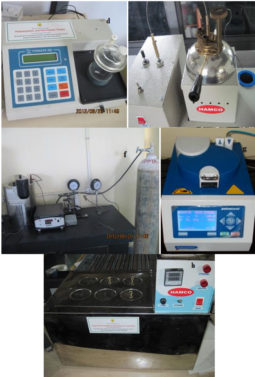
Figure 3.18 Instruments used for analysis of biodiesel properties (a). Density meter, (b), Viscometer, (c) Pour and cloud point, (d) Karl Fischer Titrator, (e) Fire and Flash point, (f) Bomb calorimeter, (g) PetroOxy for oxidation stability analysis, and (h) Copper strip corrosion method apparatus
