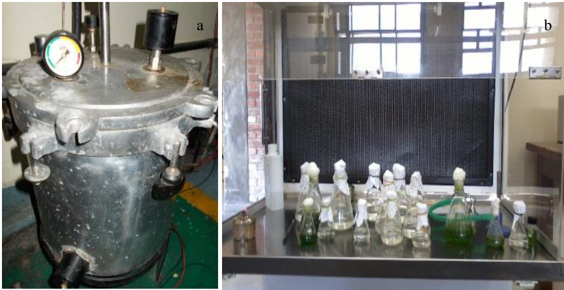
Figure 3.3 Sterilization techniques for microalgae culture, (a) autoclave for medium sterilization, (b) Laminar hood for culture transferring into new medium
