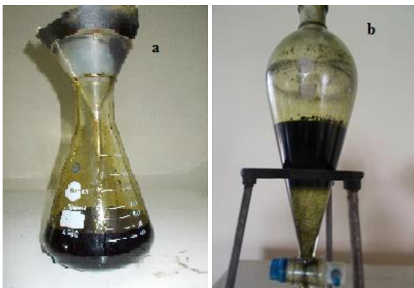
Figure 4.35 Images shown microalgae lipid and biodiesel, (a) microalgae lipid/oil, (b) microalgae biodiesel
