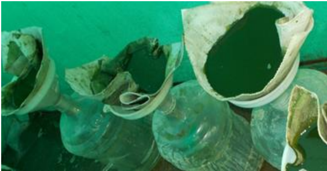
Figure 3.12 Filtration of concentrated algae slurry through filter cloth
