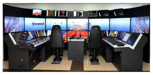
Figure 1.10 An Example set up of Full Mission Bridge Simulator(Courtesy: Bibby Ship Management)
