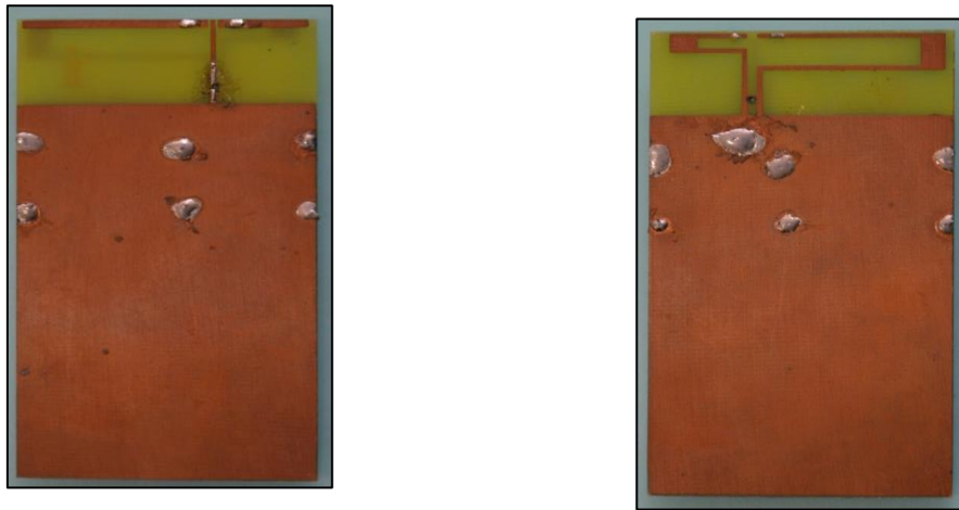
Fig 3. 13 Fabricated Antenna on FR4
