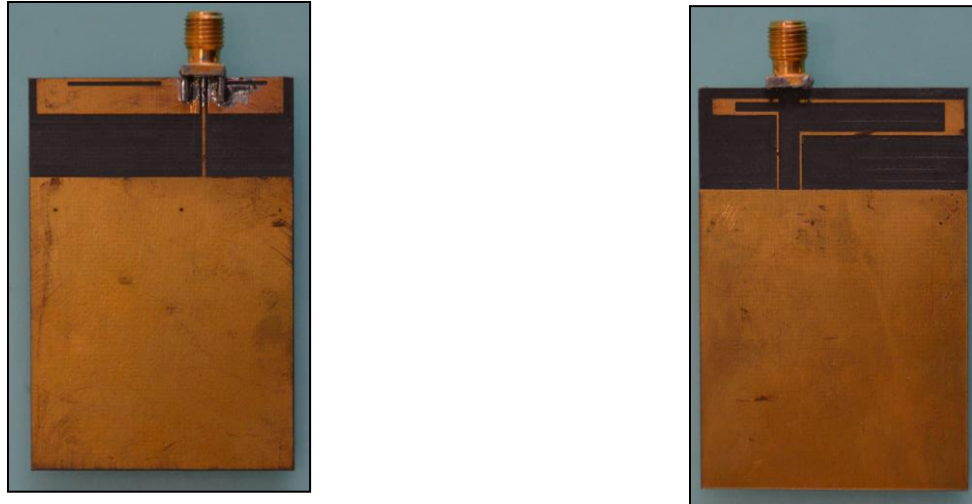
Fig 3. 15 Fabricated Antenna on RT Duroid and with slot
