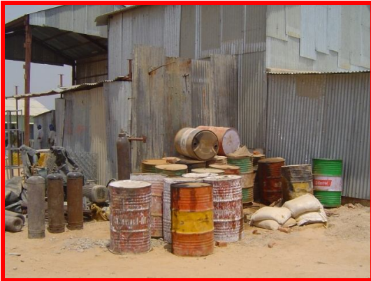
P-31: Unsafely kept cylinders & drums
